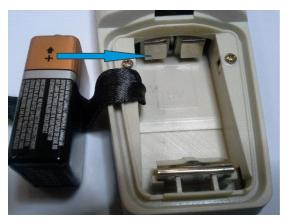
Find the 9 volt battery in the bag (USA only), remove from plastic covering. Open the battery compartment on the mindGear by sliding down the lock and lifting off the cover. Locate the + sign on the battery. Find the picture of the battery in the slot and place the battery likewise. + on battery to + terminal. Ensure that the battery is installed over linen strip to help when removing battery. Replace the cover and slide up the lock.
