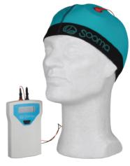
Figure 1. Sooma tDCS™ consists of a light-weight, battery-powered stimulator, electrodes with conductive medium, and a headcap with fixed electrode positions.
