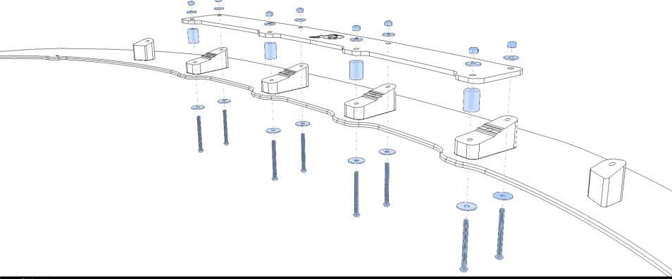
14. Using a **4mm Hex Wrench** and **10mm Wrench**, install **HARDWARE (D)** through holes **(D)** and **HARDWARE (E)** through holes **(E)** hand tight. (Pull Splash Tray down to gain access to backside)
