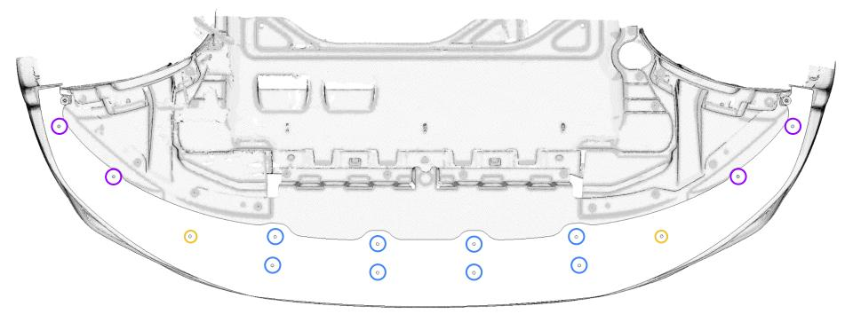
13. Using a **4mm Hex Wrench** and **10mm Wrench**, install **HARDWARE (C)** through holes **(C)** hand tight. (Pull Splash Tray down to gain access to backside) NOTE: **[Order of fasteners/parts from bottom to top - Bolt, Fender Washer, Splitter, Bumper, Spacers, aerobrace, 18mm Washers, Lock Nuts.]** Install and hand tighten only one set of fasteners at a time. This will allow for more room to work with. \*NOTICE SPACER ONLY INSTALL AT REAR HOLES\*
