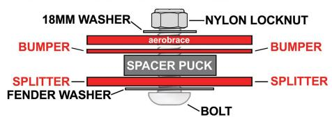
\*aerobrace installs on topside of bumper followed by 18mm washer and locknut.
