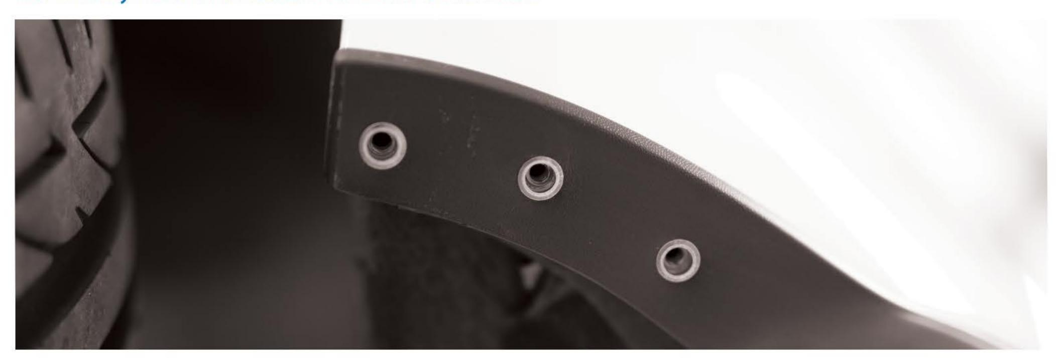
10. With **Rivnuts** installed, loosely install Spats using **HARDWARE** (**B**) and align the pre-drilled holes (**C**) with your **Rivnuts**. Using a **5/32**" **Hex Drive** and **Medium-Threadlocker**, install **HARDWARE** (**C**) through holes (**C**) and into **Rivnuts**. Tighten **HARDWARE** (**C**) until snug/Spats sit flush with Valance. Fully tighten **HARDWARE** (**B**) and repeat on opposite side.
