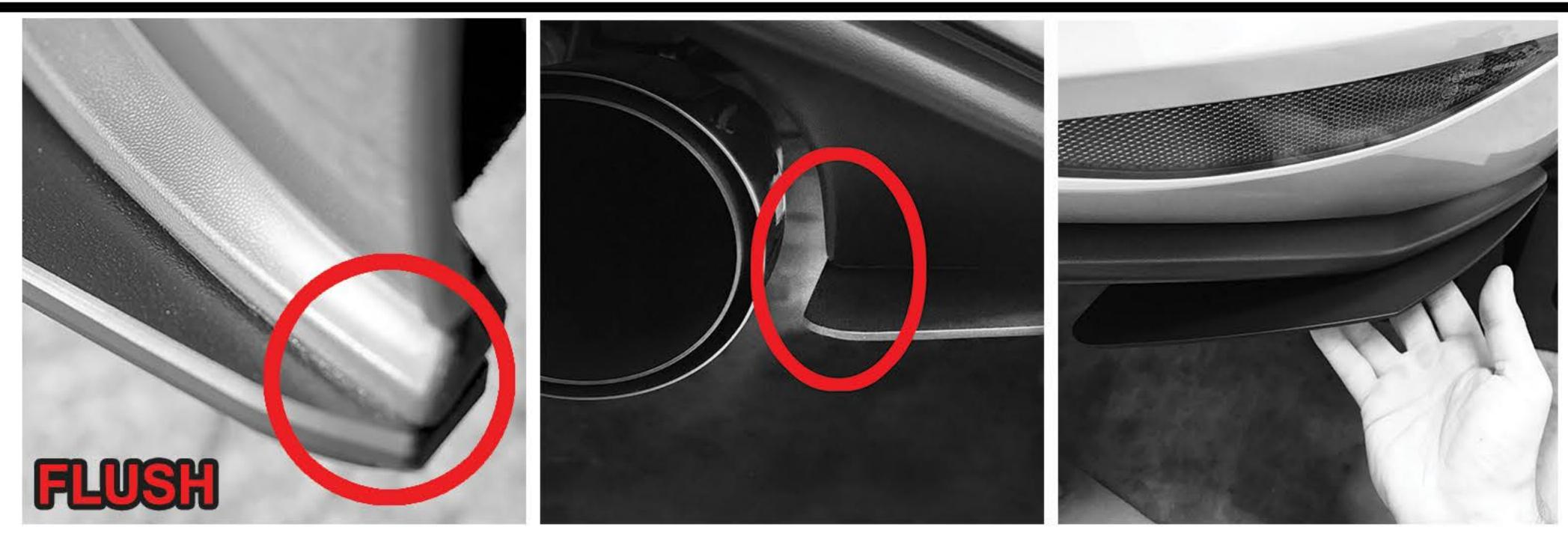
2. With the Side Spat aligned, use a **Light Colored Marking Tool** to mark through the pre-drilled holes onto bottom side of Factory Valance. Remove Spat. **-IMPORTANT:** As shown below, markings on surface should be placed in center of ledge.
