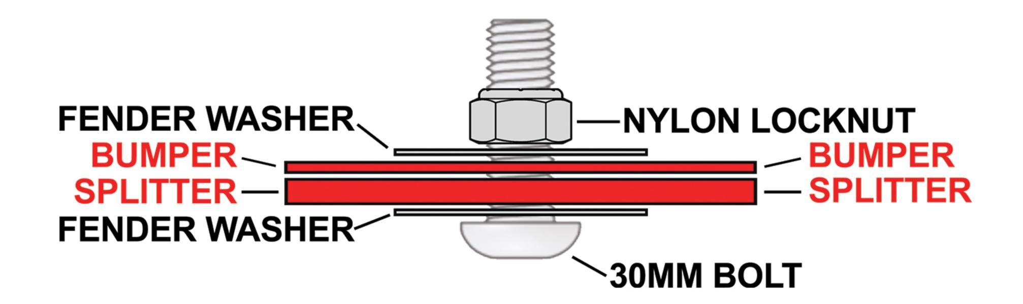
12. Using a 4mm Hex Wrench and 10mm Wrench, install the aerobrace™ with the hardware from HARDWARE (C). Fasten Splitter to Bumper by passing through Splitter holes (C) in the order shown on right and tighten. (Pull Splash Pan down to gain access to backside)
