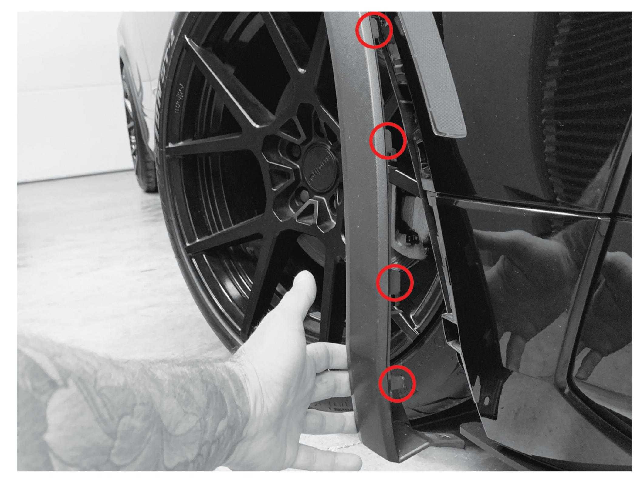
5. Pull away Fender Liner from Bumper. Identify and remove the factory Clip-On Nuts used for fastening the Fender Arcs attached to bottom of Liner.
