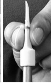
Squeezing the belt-wire at the flat surfaces of the reed blades will reduce the reed opening.
