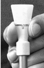
Squeezing the reed at the two belt-wire edges will increase the reed blade opening.
