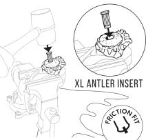
Find a solid surface to mount your **XL Antler Bar**. This Antler Bar can be installed into a flat surface or vertical surface. (Optional: Use a drill with a 3/8" or 7/16" bit to pre-drill a hole into the desired surface). Use a 1/4" Hex driver to install the XL Antler Bar. (If you're installing it to drywall, be sure to fasten the product to a stud for a secure mount).
