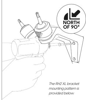
For added strength and security, use the provided 3/16" hex wrench to tighten the set screw located on the bottom side of the bracket. This screw will lock the ball joint assembly in your desired position.
