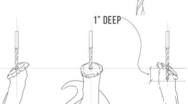
An improperly drilled hole may result in the need to add an adhesive to the antier insert.
