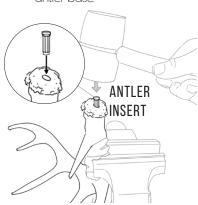
Slide the antler onto the hex end of the Antler Bar by aligning the bar with the Antler Insert (mating hex features). Slide the antler down until it's fully engaged on the Antler Bar. Now you can tighten the Antler Bar slightly if needed to adjust your angle. Note: Because this is a hex feature, you have six sides of antler angle adjustment.
