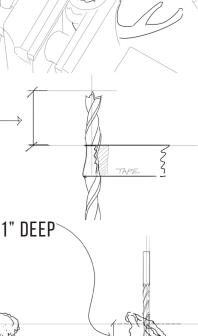
Starting with the small end, place the antler insert into the drilled hole. Press the insert in until it's snug, and then find a rubber mallet. Using the mallet, gently tap the insert into the antler until the top lip of the insert touches the antler base.
