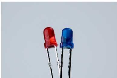
Blue and red LEDs Note: long leg is positive
