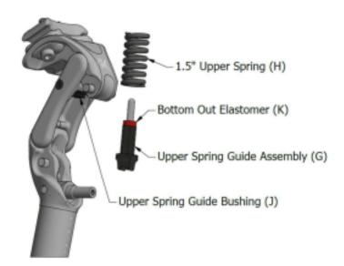
Install upper spring assembly by inserting the top first into the Upper Spring Guide Bushing (J), and then push the bottom into place over the stainless pivot pin.
