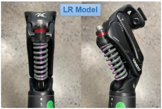
All XR/Body Float XL/2XL have an upper 1.5" spring and a larger 2" lower spring. The lower side links will connect/wrap around the preload bolt. Below is an example of the springs and the lower side links.
