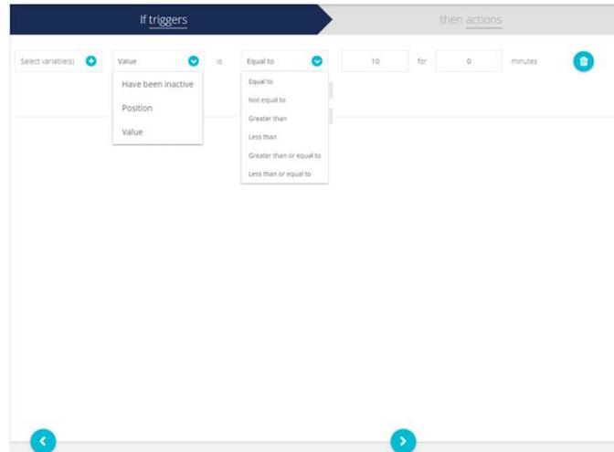
This page lets you set up the **trigger(s)** for the event. You select the variable and how it triggers. You can have multiple and/or triggers. Click the right arrow to move to the next page.
