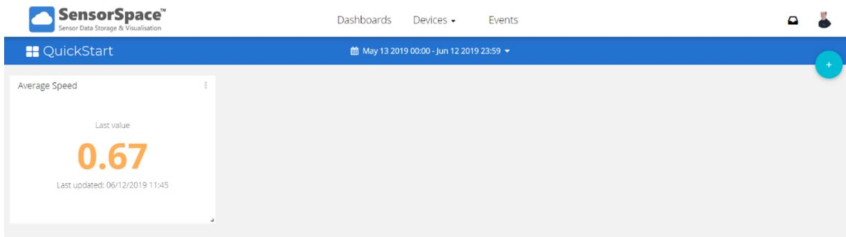
We can resize the widget by grabbing the bottom right corner. Move the widget to where you want on the screen by clicking and holding the top of it. Clicking the three dots in the top right of the widget allows you to **Download** the widget's data, **Share** the widget via a weblink, **Edit** the settings or **Delete** the widget. Note: deleting the widget does not delete the data, this is fed from the Device(s).
