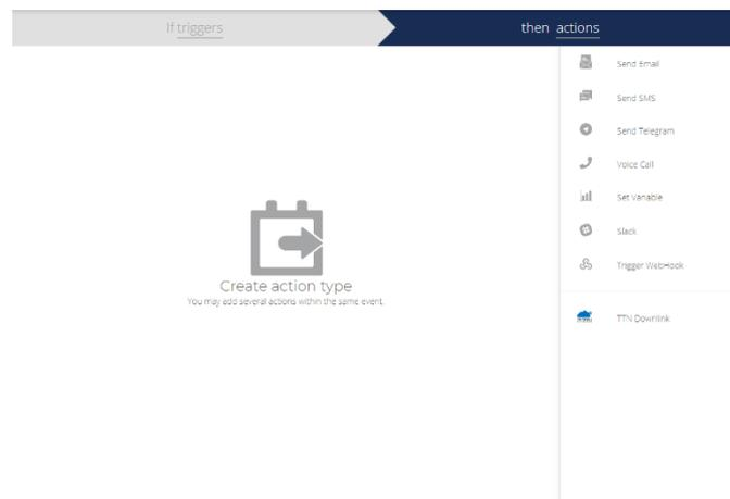
Here you select the action type then fill in the relevant parts. This includes setting the message contents using text and the **Custom Fields** to reference variables and times etc.
