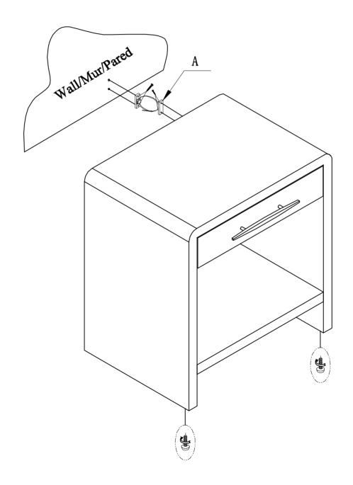
Adjust levelers if needed, to level case on uneven floor
