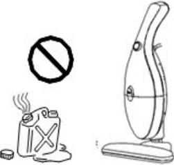
A line drawing of the Handi Vac unit on the right. To its left is a gas can with a flame. A circular prohibition sign with a diagonal slash is placed over the flame, indicating that the device should not be used to clean flammable substances.                               |
