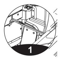
Installing the calf rest, unfasten the fixed pipe belt and insert the connecting part into the seat frame.
