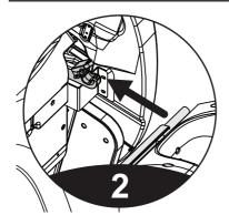
Clip in the round metal tube from calf rest into the left and right side clips
