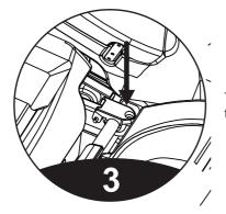
Turn the leg fixing cover over the round tube on both sides of the legs (figure 3)
