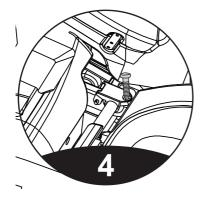
Use 2pcs M4 screws to fix the legs to the massage chair. Check thoroughly that the wires and air hose are properly connected and manually check the calf section can move freely.
