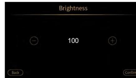
Please set up the brightness of coffee machine according to the following steps:
