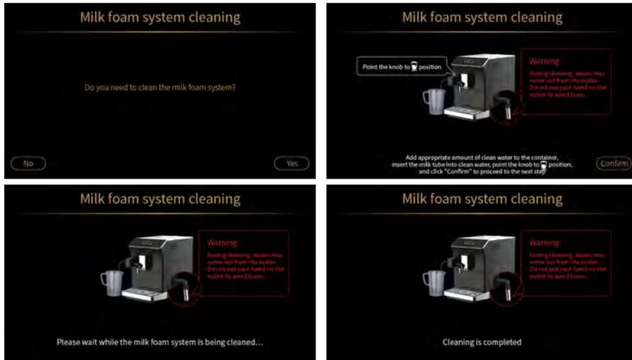
The Cleaning process of Milk Foam System:
