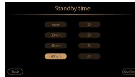
The factory setup of the machine is that the machine will automatically start cleaning and then enter standby mode if not used continuously for 60 minutes. You can set to turn off the machine automatically 30 minutes, 45 minutes, 60 minutes, 2 hours, 3 hours, 4 hours and 5 hours after using it.
