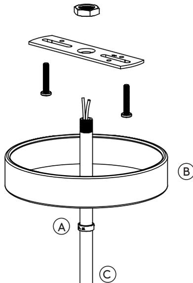
4. Loosen the set screw on the slip ring (A) and lower with canopy (B) gently down the drop stem (C).
