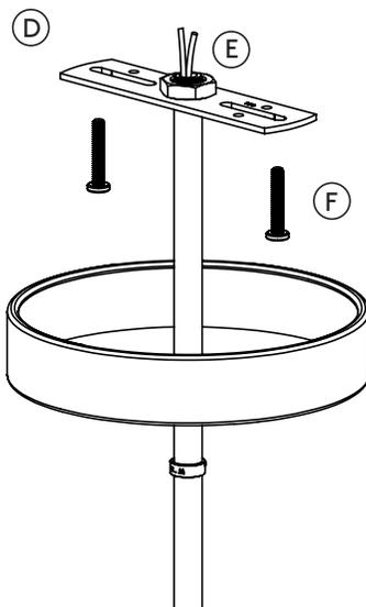
6. Screw on the cross bar (D) to the top end of the threaded drop stem with the nut (E).
