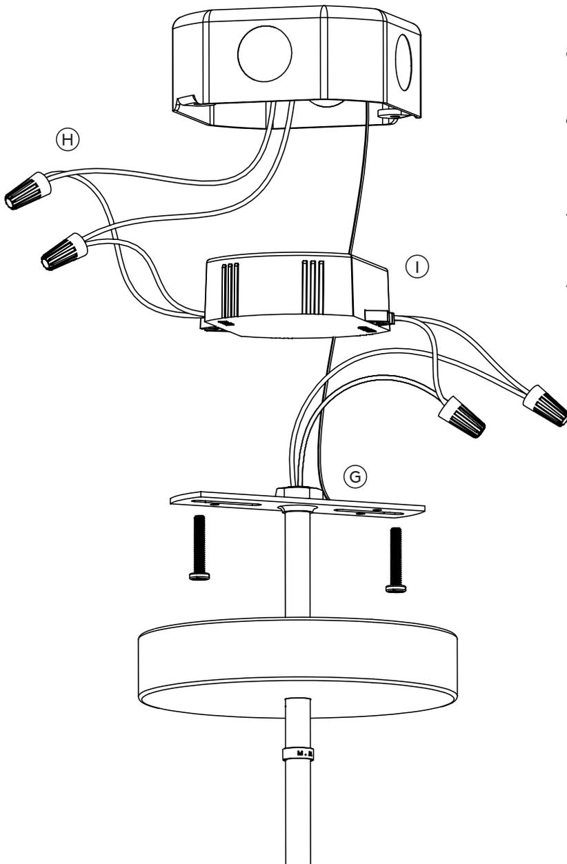
NOTE: The drawing is exploded for illustrating wiring and electrical connections.
