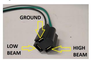
Light Pink ( labelled -24 Left Low Beam ) ( 16awg ) wire to black three pin headlight plug supplied with this kit along with the headlight ground wires to the connectors as per above diagram
