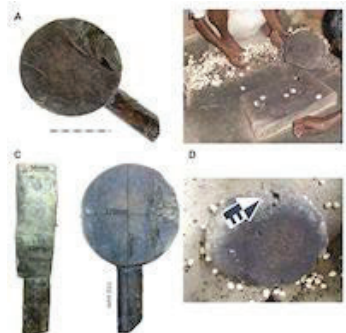
Figure 8: Hammer and anvil used for popping the dried and roasted E. ferox nuts in traditional practices in Madhubani District, Bihar, India: (A) General view of a wooden hammer ( Thaapi ) (photograph: Gabi Laron); (B) A wooden anvil ( Aphara ); (C) Measurements of a typical hammer; (D) Close-up of an anvil used for popping E. ferox nuts. (Image credit: authors)
