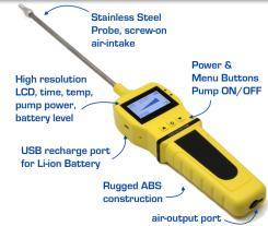
PUMP ON / PUMP OFF: When power up, pump will turn ON. The screen shows temp, time & battery level. A large triangle represents the pump power. If pump load is detected that slows down the pump flow, the triangle power level will reduce accordingly. Quickly press POWER button to turn ON/OFF the pump. When the PUMP is OFF, the RED LED with FLASH.
