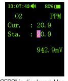
save. When complete, "SAVE SUCCESS" is displayed. Use an appropriate multigas mixture is OK or single gas mixture is also OK to calibrate a single sensor.
