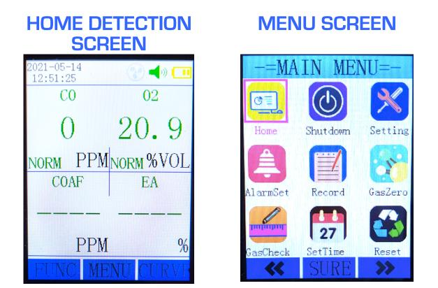
The analyzer calculates COAF (CO Air Free) and Excess Air (EA) only when the O2 reading is less than 20%
