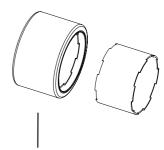
The rear tires have an internal metal ring, it will prevent the vibration during riding.
