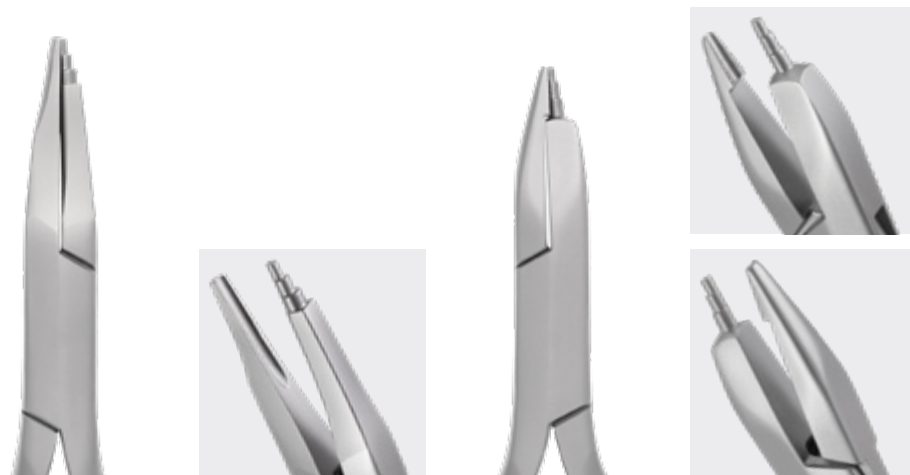
3000/96 Tweed – Long ø max 0,5 mm / .020" (mm 145) Designed to form precise omega loops. Long grooved beak internally smoothed. Long type. 3000/97 Tweed – O'Brein ø max 0,7 mm / .028" (mm 140) Graduated cone to form precise omega and closing loops. Micro serrated beaks to prevent wire slippage.
