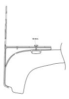
8. Fit awning to awning mount using the bolts provided with awning and tighten to specs within awning instructions.
