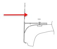
15. Fit awning to bracket using the bolts provided with awning and tighten to specs within awning instructions.
