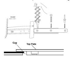
13. Fit top plate with one bolt (M6x10mm) at each end, these bolts will hold the top plate when the Rackless awning mount system is not installed.
