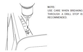
7. Use a vacuum to remove swarf from the roof channel.
