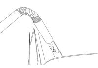
8. Apply anti rust paint to the inside and surrounds of all holes, allow for time to dry before applying silicon around each hole and along the mount length.
