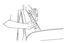
7. Marked out holes can now be drilled using a 5mm drill bit with a drill stop. Set up the drill stop ensuring you don't drill through the roof lining.
