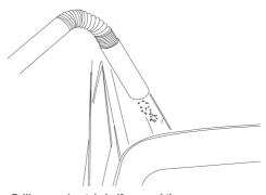
Drill approximately halfway and then use a vacuum to remove swarf from roof channel. Continue drilling the hole, repeat operation for remaining holes.
