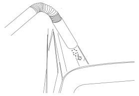
Drill approximately halfway and then use a vacuum to remove swarf from roof channel. Continue drilling the hole, repeat operation for remaining holes.
