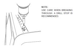
8. Use a vacuum to remove swarf from the roof channel.
