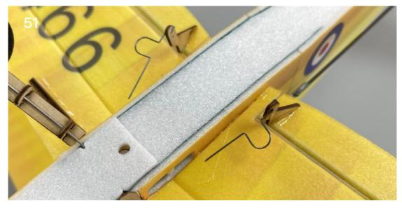
52. Attach the steel wire clips to the aileron servo arms. Connect the steel wire hooks and wire clips with heat shrinkable tubes.
