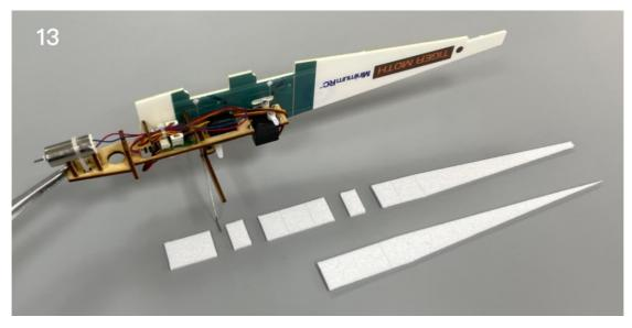
14. Fix the top and bottom strip of the fuselage with glue.
