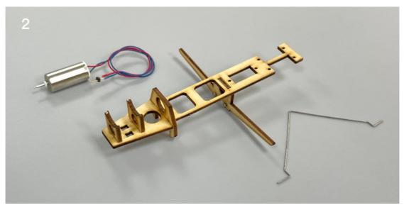
3. Fix the landing gear steel wire with m1x3 screws.
