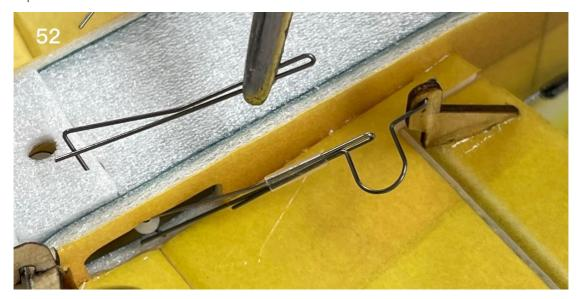
53. Connect the aileron steel wire hooks and clips with heat shrinkable tubes on both sides.
