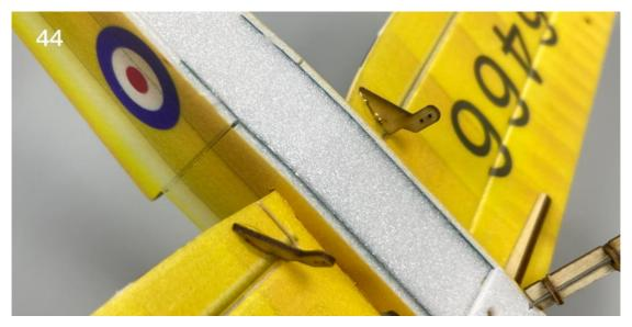
45. Install rudder and elevator control horns.
