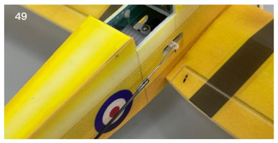
50. Cut the carbon rod to proper length and connect the wire hooks with heat shrinkable tubes.
