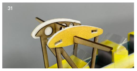
32. Bend the fuel tank cover along its shape.
