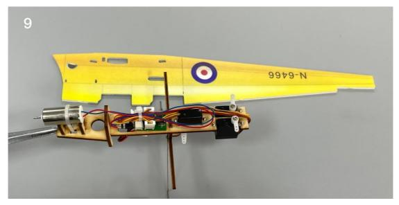
10. Align the scribed line on the inner side of the fuselage and fix the wooden structure with glue.
