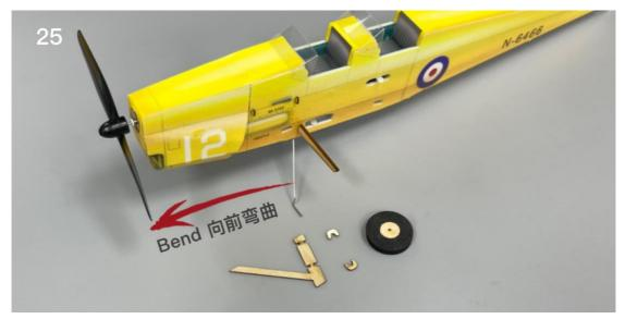
26. Install the landing gear cover plate and wheels. Bend the outer end of the steel wire with pointed nose pliers.
