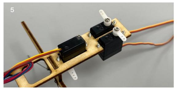
6. (Bottom view) The three servos are installed and fixed under the plywood board.
