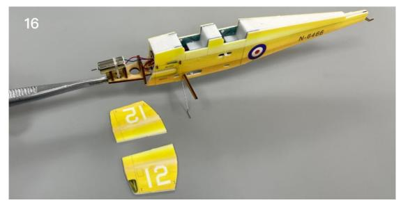
17. Install nose cover on one side. Note: the position shown in the picture is the battery cover plate that can be opened. No glue shall be applied to the area marked by the yellow line.
