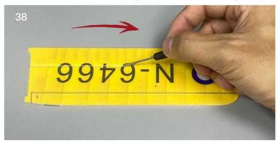
39. Use the end of a screw driver to score through the aileron half-cut line of the aileron.
