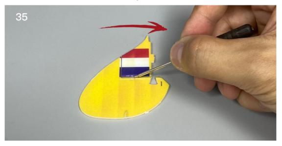
36. Use the end of a screw driver to score through the aileron half-cut line of the horizontal tail.
