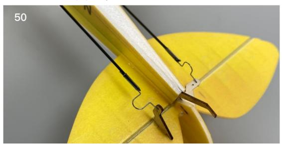
51. Attach the steel wire hooks to the aileron control horns.
