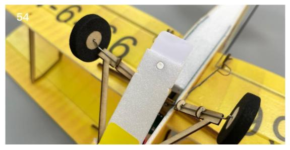
55. Fix the battery cover magnet with glue and cover it with stickers.
