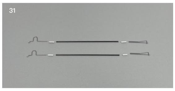
32. Use heat shrinkable tube to connect the pull rod and wire clip, then use glue to fix them.
