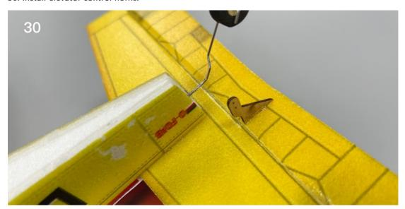
31. Use heat shrinkable tube to connect tail push rod and steel wire clip.
