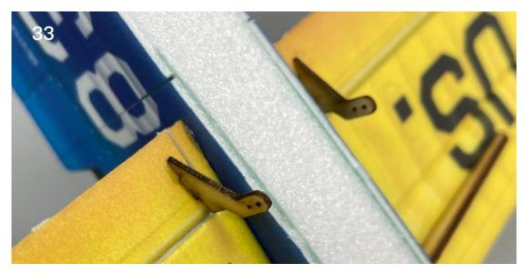
34. Install rudder and elevator control horns.
