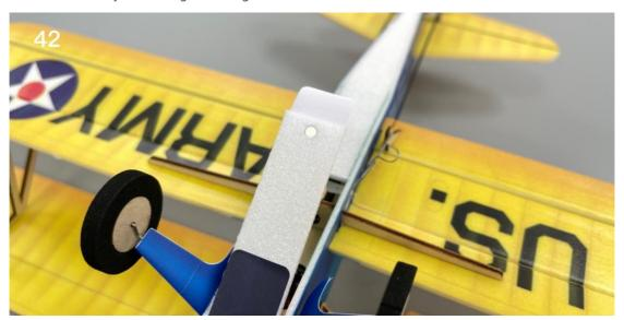
43. Fix the battery cover magnet with glue and cover it with stickers.
