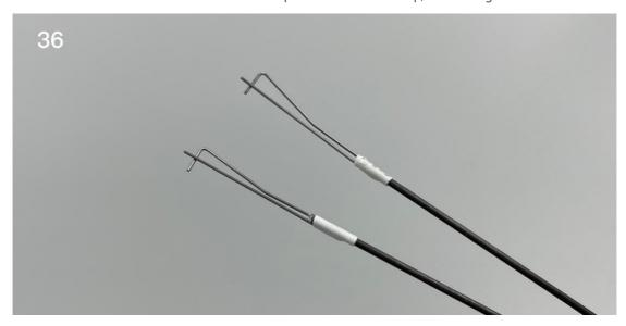
37. Attach the steel wire hooks to the control horns.
