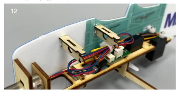
13. Note: the position shown in the picture is the battery cover plate that can be opened. No glue shall be applied to the area marked by the yellow line.
