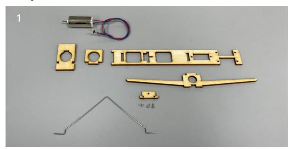
2. Bond the plywood structure with CA glue. Fix the landing gear steel wire with m1x3 screws.
