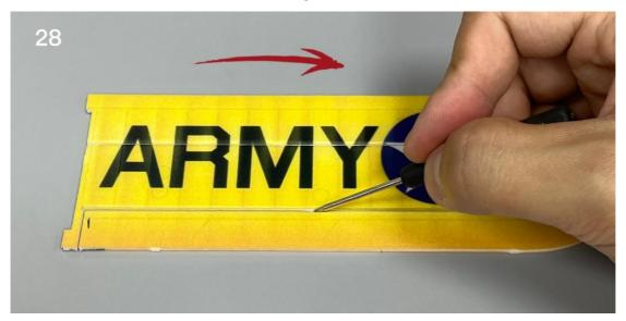
29. Use the end of a screw driver to score through the half-cut line of the upper wing surface.
