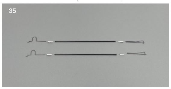
36. Use heat shrinkable tube to connect the push rod and wire clip, then use glue to fix them.
