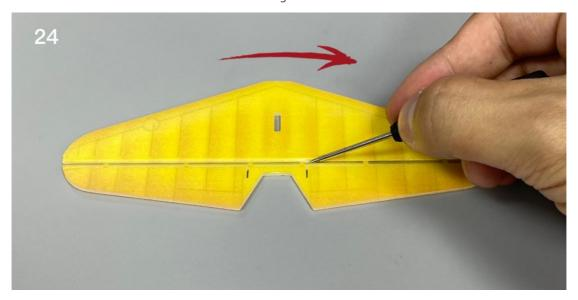
25. Use the end of a screw driver to score through the aileron half-cut line of the vertical tail.
