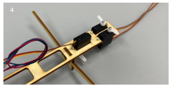
5. (bottom view) The three servos are installed and fixed under the plywood board.
