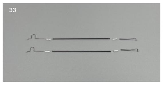
34. Use heat shrinkable tube to connect the push rod and wire clip, then use glue to fix them.
