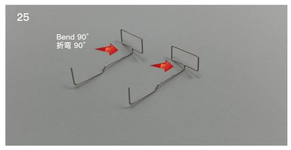
26. Bend the outer end of the steel wire with pointed nose pliers.
