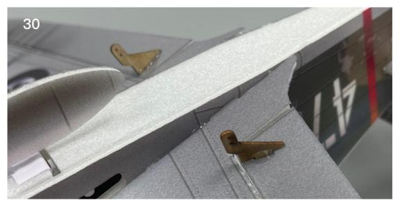
31. Install rudder control horns.
