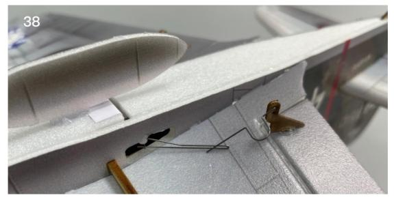
39. Connect the steel wire hooks and wire clips with heat shrinkable tubes.
