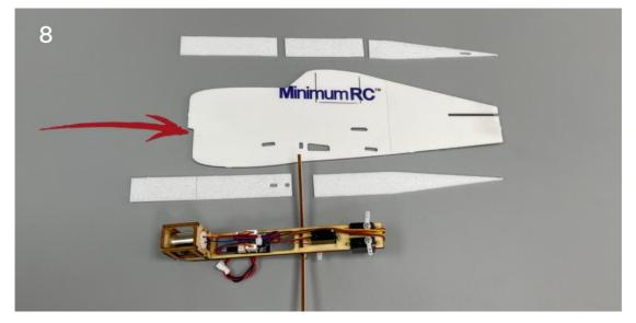
9. Align the scribed line on the inner side of the fuselage and fix the wooden structure with glue.
