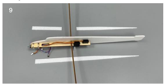
10. Fix the top and bottom strip of the fuselage with glue.
