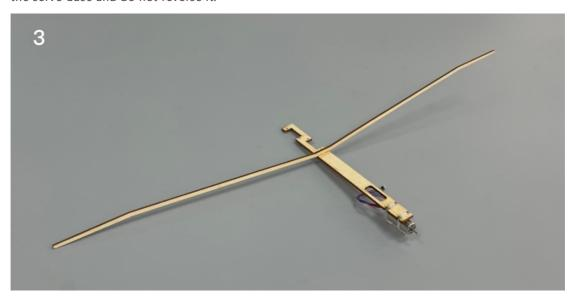
4. fix the motor with a tie, and the fixed end of the tie should be just at the bottom. After fixing, 502 glue shall be applied to the side for reinforcement.
