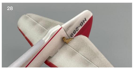
29. Attach the steel wire hook to the control horns.
