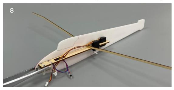
9. Press the top and bottom strip of the fuselage and bend them into the corresponding shape of the fuselage.
