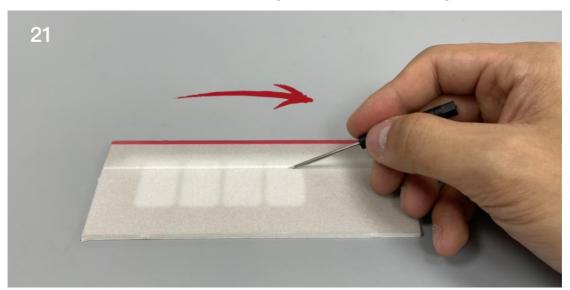
22. Use the end of a screw driver to score through the half-cut line of the wings.
