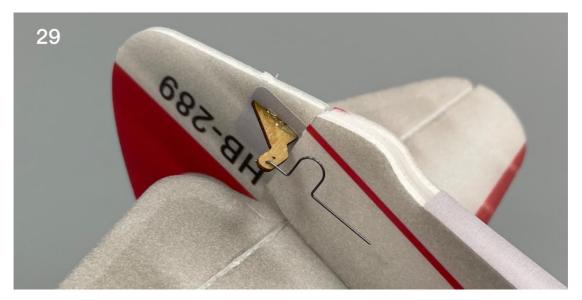
30. Attach the steel wire hook to the control horns.
