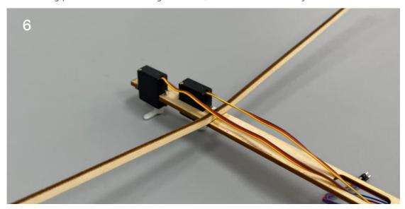
7. (bottom view) The servos are installed and fixed under the plywood board.
