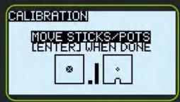
move all the gimbals, knobs, and side sliders to their respective maximum and minimum positions, and then press the ENT key to complete the calibration
