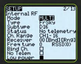
The default value of Frequene is "0". If the receiver does not bind, we can change the value to either +30 or -30 and try to bind again. If binding is still unsuccessful, continue to try higher and lower values in steps of plus or minus 30 until the bind succeeds.
