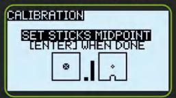
place all the gimbals, knobs, and side sliders in the middle position, and then press the ENT key
