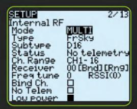
Frequency tuning. Certain protocols require tuning for optimal performance. In some cases, tuning is required in order for the protocol to bind. Frequency Tuning is specific to each MULTI-Module, and is due to very small variations in the RF components.
