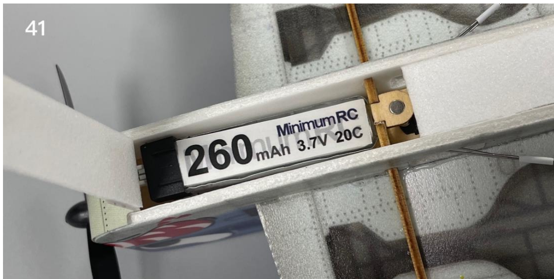
41. The battery is directly placed in the battery compartment.
