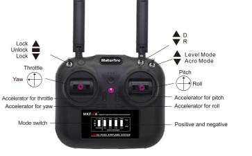
Output switch: D: the channel output value: 1150-1850(recommend for beginner). R: the channel output value: 1000-2000. Accelerator switch: Adjust the middle point of the channel.
