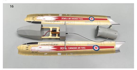
17. Use a sharp tool (screwdriver) to score through the marked lines on the fuselage.
