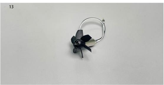
14. Assemble the motor with the duct component, adjust the motor installation depth, ensuring that the propeller blades are as close to the support structure as possible and rotate freely.(Failure to position the blades close to the support will significantly decrease thrust.) Use glue to secure the motor from the rear end, as shown in the diagram.
