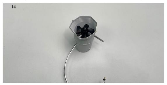
15. Connect the motor to the receiver and test it to confirm that the motor rotation direction is correct.
