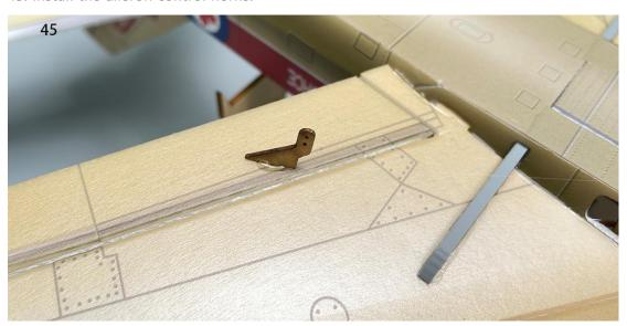
46. Install the elevator control horns.
