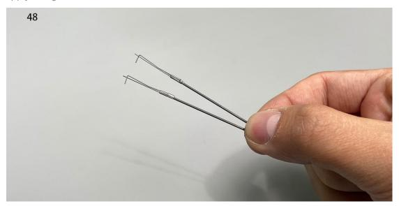
49. Install the connection hooks on the aileron control horns.
