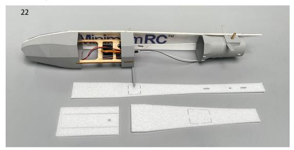
23. Secure the top PS foam board with glue.
