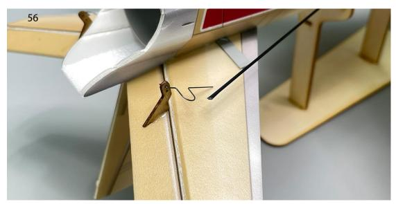
57. Use heat shrink tubing to connect the control rods to the connection hooks, then apply 502 glue for fixation.
