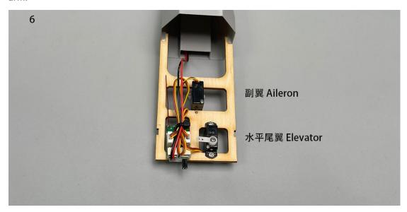
7. The aileron servo uses a cross-shaped arm.
