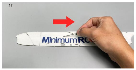
18. Caution: When performing scoring operations, make sure to press on the part closest to the lines to avoid tearing the components. (As shown in the diagram.)
