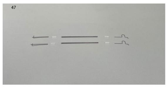
48. Use heat shrink tubing to connect the control rods and servo wire clamp heads, then apply 502 glue for fixation.
