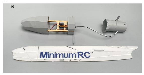
20. Assemble one side of the fuselage, the wooden framework, and the duct with glue.
