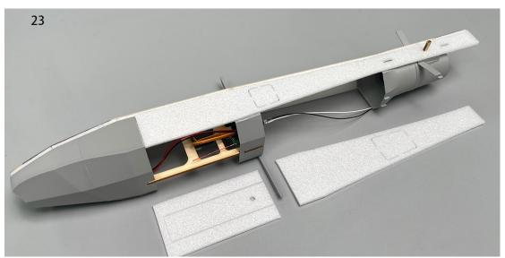
24. Use glue to secure the bottom PS board, being careful not to apply glue to the battery cover.
