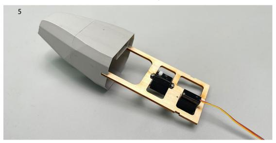
6. Secure the receiver with Velcro. Connect the receiver to the servos and bind the receiver with the transmitter. Test whether the servos are functioning properly, ensuring that the servos' correspondence with the channels are correct. Install the elevator servo arm.
