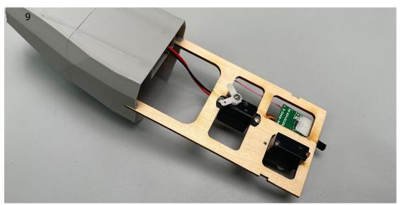
10. Install middle section support component of the fuselage.
