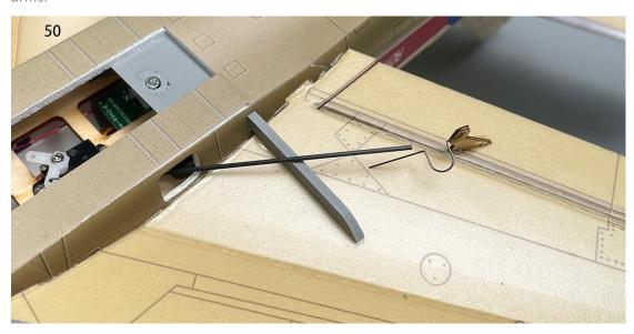
51. Use heat shrink tubing to connect the aileron control rods to the connection hooks, then apply 502 glue for fixation.
