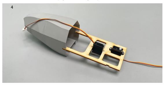
5. Install the servos as shown. (Bottom view of the parts.)
