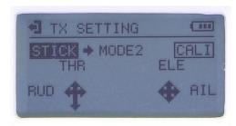
B. Select "CALI", long press to enter the remote rod calibration page, SET the remote rod in neutral position, then select "SET" and short press to circle the remote rod to the maximum extent. Once completed, short press "SET" again.
