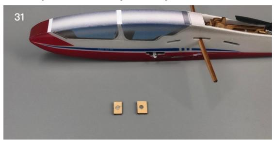
32. Install the fuselage magnet seat.
