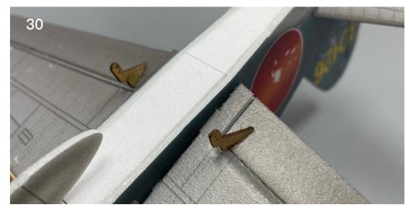
31. Install rudder control horns.
