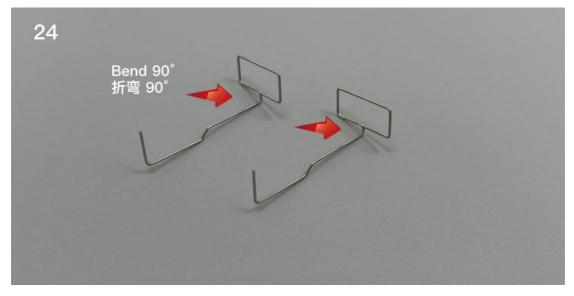
25. bend the outer end of the steel wire with pointed nose pliers.
