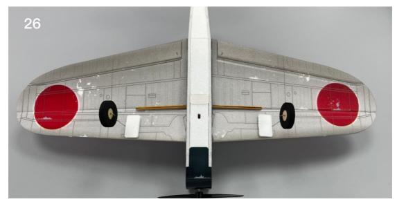
27. Fix the landing gear cover plate with circular stickers, which can be reinforced with glue.
