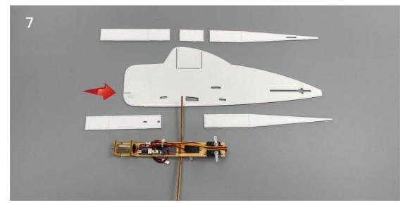
7. Align the scribed line on the inner side of the fuselage and fix the wooden structure with glue.
