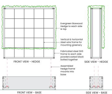
WPC panels to each side Galvanised steel fabricated corner brace bolted into each corner **BOTTOM VIEW - BASE**
