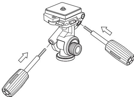
Panhandle are installed as shown. There is not difference in length between the panhead, and screw into the back of the pan & tilt handle.
