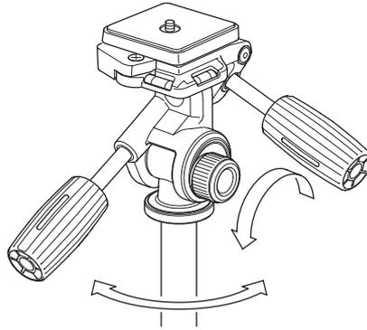
Loosen the panning lock knob, and the head will rotate along the horizontal direction.
