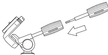
Remove the vertical tilt handle from the panhead, and screw into the back of the pan & tilt handle.
