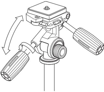
Loosen the pan & tilt handle, and the head will tilt back and forth.
