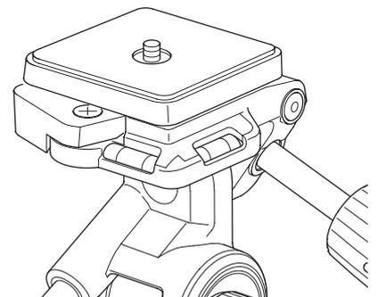
Adjust the built-in level to fit into the middle.
