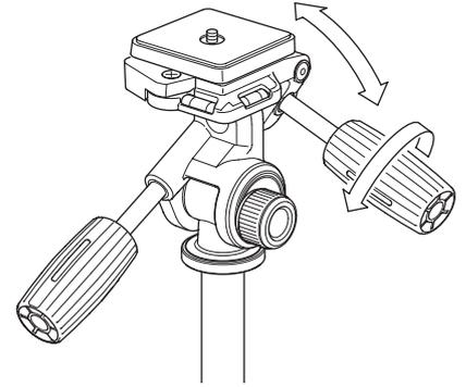
Loosen the vertical tilt handle, and the level can be adjusted.
