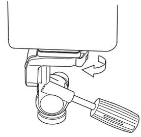
When you fix this quick release platform to pan head, the quick release lock lever will return to the original position automatically. We, however, recommend you to tighten this lever more to secure the fixing.
