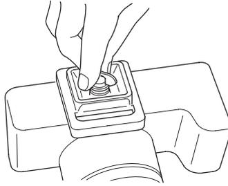
Align the length of the platform along the base of the camera body, and securely tighten the mounting wing nut.
