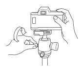
By turning the tension adjustment knob (located opposite of the ball locking knob), you can adjust the tension of the ball movement. Make sure to hold your camera while operating the tension adjustment knob. Make adjustments after loosening the locking knob slightly, so as to free the ball movement.
